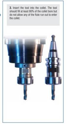
Note: To ensure trouble free operation, always insert the collet into the collet nut until it clicks in and thread it loosely onto the spindle prior to inserting router bit.
